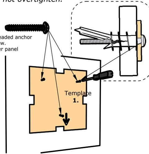
**4. Insert Template 2. into next required face on Template 1 & repeat 1&2. To add additional panels remove the template to be moved, repeat the process until the layout is completed.**
