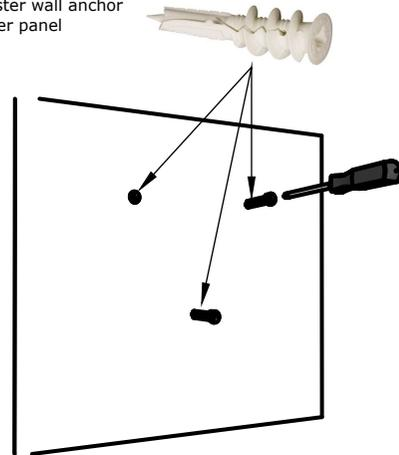
**3. To install additional panels reposition Template 1. & insert screws until firm. Do not overtighten.**
