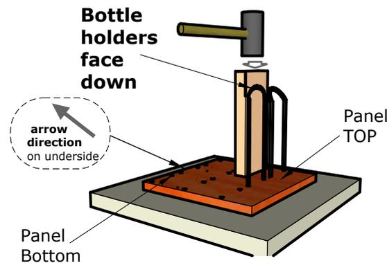
**7. Commencing with the lowest panel position, align the panel with the panel connectors, push in & pull down.**
