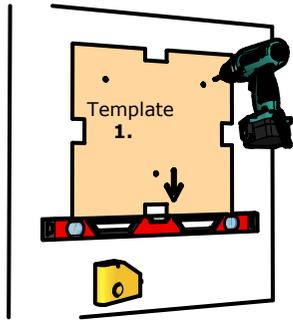
**2. Screw in wall anchors until flush. Do not overtighten. If installing single panel go to 5.**
