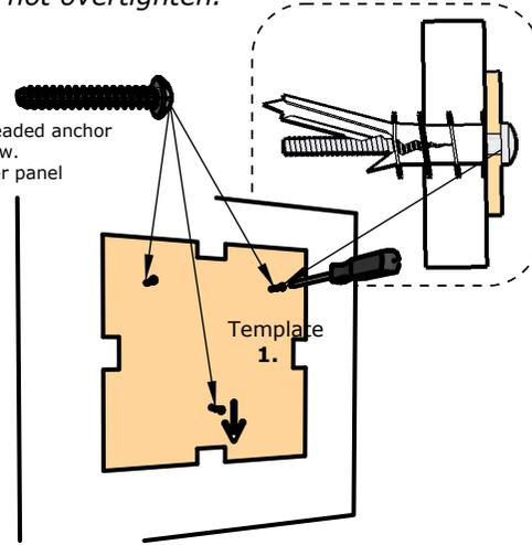
**4. Insert Template 2. into next required face on Template 1 & repeat 1&2. To add additional panels remove the template to be moved, repeat the process until the layout is completed.**
