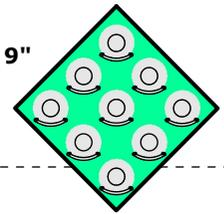
**1. Mark the layout dimensions on the wall, select a corner starting point, Position & accurately level Template 1. Drill the 3 Template holes, 4.2mm drill bit supplied. Ensure the template does not move thru the process.**
