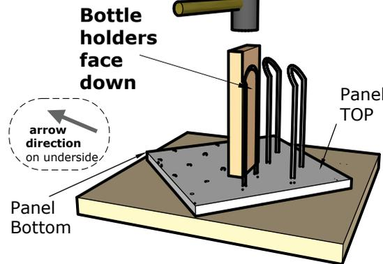
**7. Commencing with the lowest panel position, align the panel with the panel connectors, push in & pull down.**
